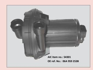
directly behind the valves in the exhaust manifold. Because of the secondary air injection, the catalytic converter is brought to operating temperature more quickly — which leads to a reduction in pollutant emissions. The automatic recirculation valve (ARV) has the task of preventing exhaust or condensation entering the secondary air injection pump.
